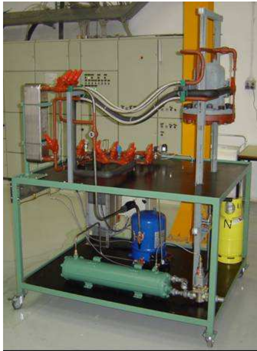
Figure 4.13: Front picture of Marine Chiller System
