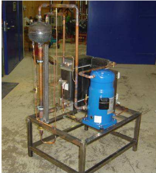
Figure 4.11: Front picture Heat Pump System for milk cooling
