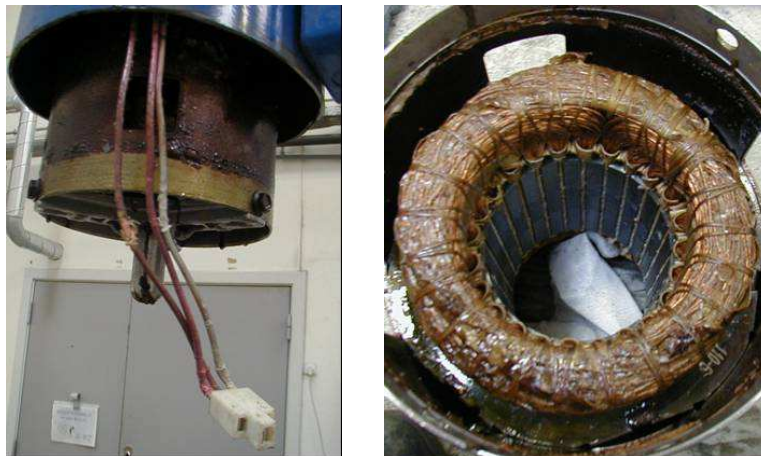
Figure 5.8: Pictures from investigation of the damaged scroll compressor
