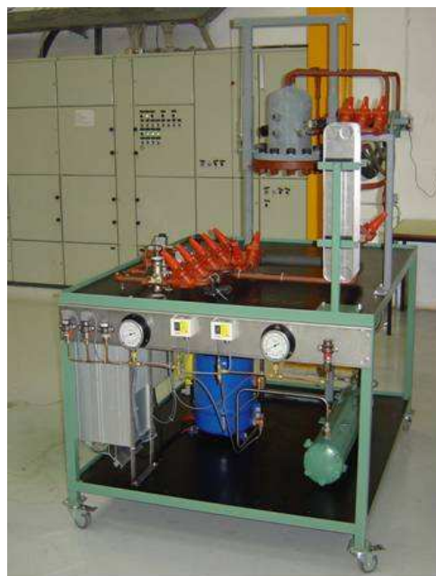
Figure 4.12: Front picture of Marine Chiller System
